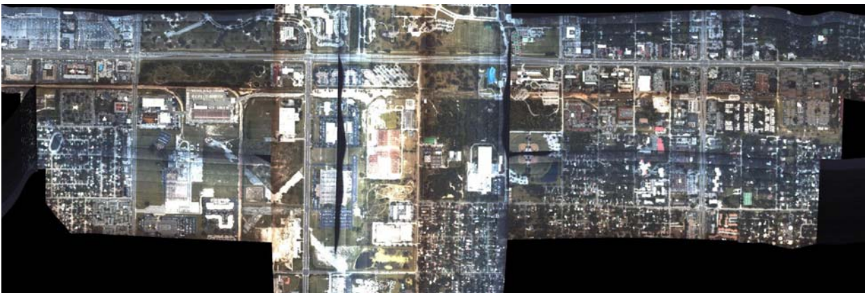
Figure 3.7: Mosaic of 6 hyperspectral flightlines as processed with PARGE. (© Florida Environmental Research Institute's Spectroscopic Aerial Mapping System with Onboard Navigation (SAMSON) sensor)
