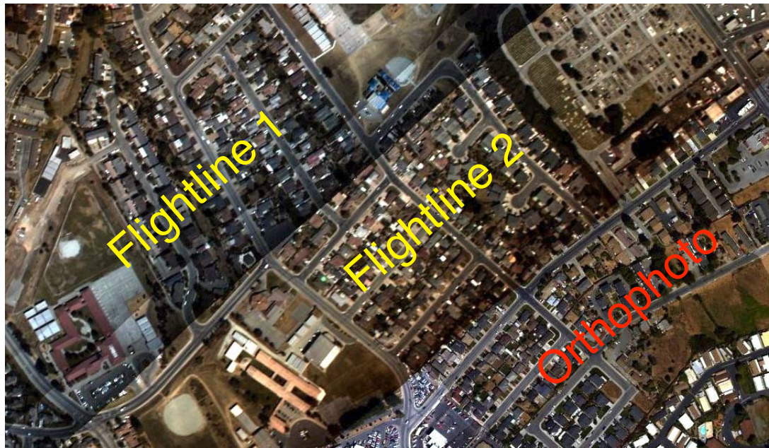
Figure 3.8: Overlay of two SAMSON flightlines with a digital orthophoto at 1 m spatial resolution
